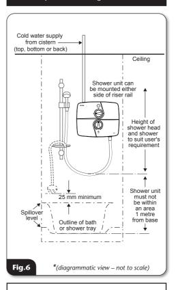
**IMPORTANT:** If installing onto a tiled wall, **ALWAYS** mount the unit on the surface of the tiles. **NEVER** tile up to the unit.
