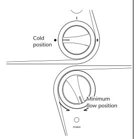
\*IMPORTANT: Failure to turn the temperature control to the minimum flow position may cause the PRD to operate.
